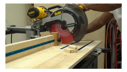
Use the **stop block** for repeatable cuts. You can cut up 32 inches, feel free to make this longer i needed.
